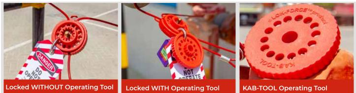
The innovative **Operating Tool** can be locked into the base unit with a padlock. When multiple valves have to be isolated, the Operating Tool locks into the last valve ensuring availability of Tool on hand during the re-energization process.
